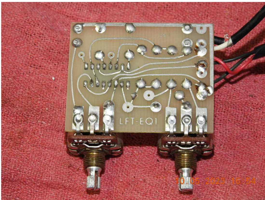
LFT-EQ1 PreAmp Board, Circa 1984 (mounted pots, solder side)
