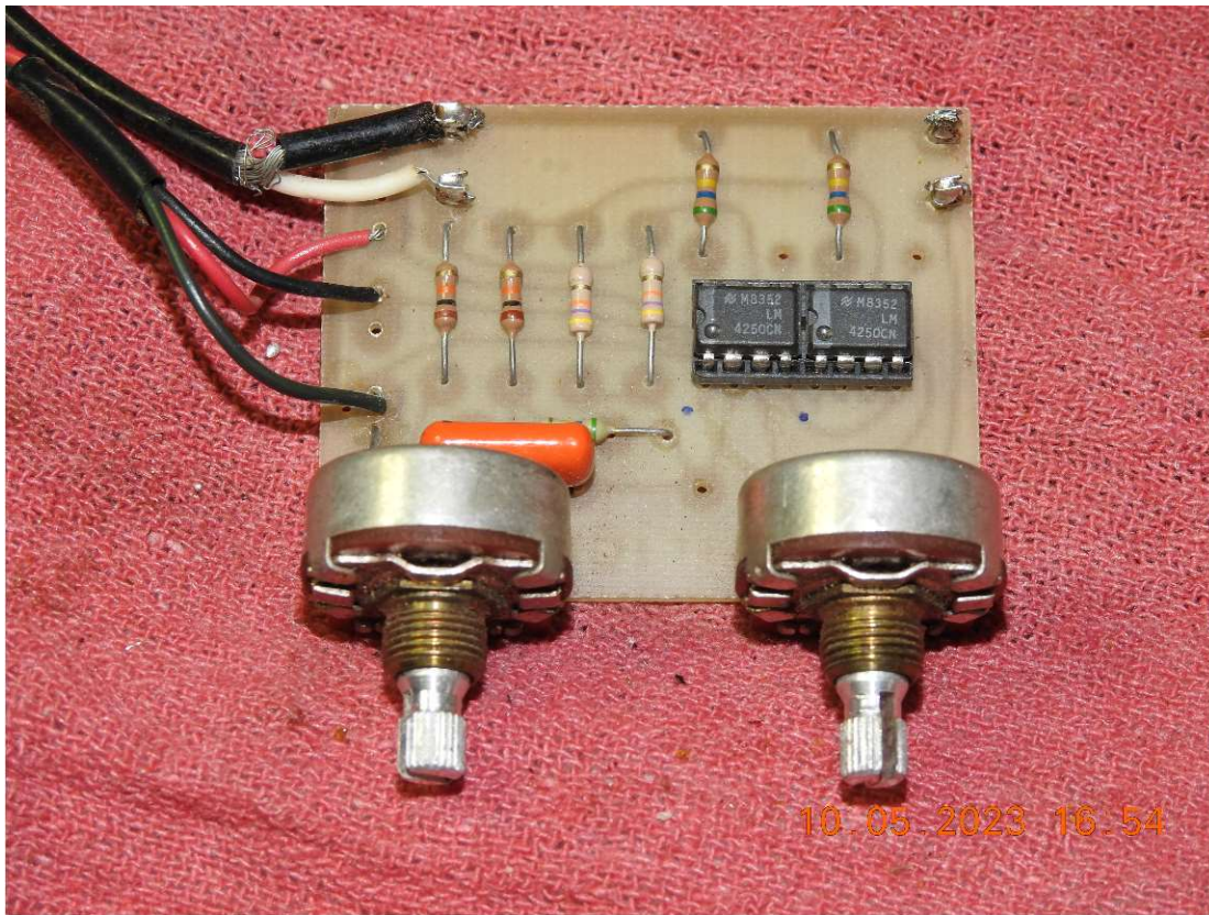
LFT-EQ1 PreAmp Board, Circa 1984 (mounted pots, solder side)
