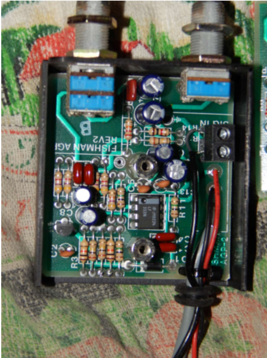
Fishman AGP-2/ABGP-2 PreAmp Board, Circa 1990 (component side)
